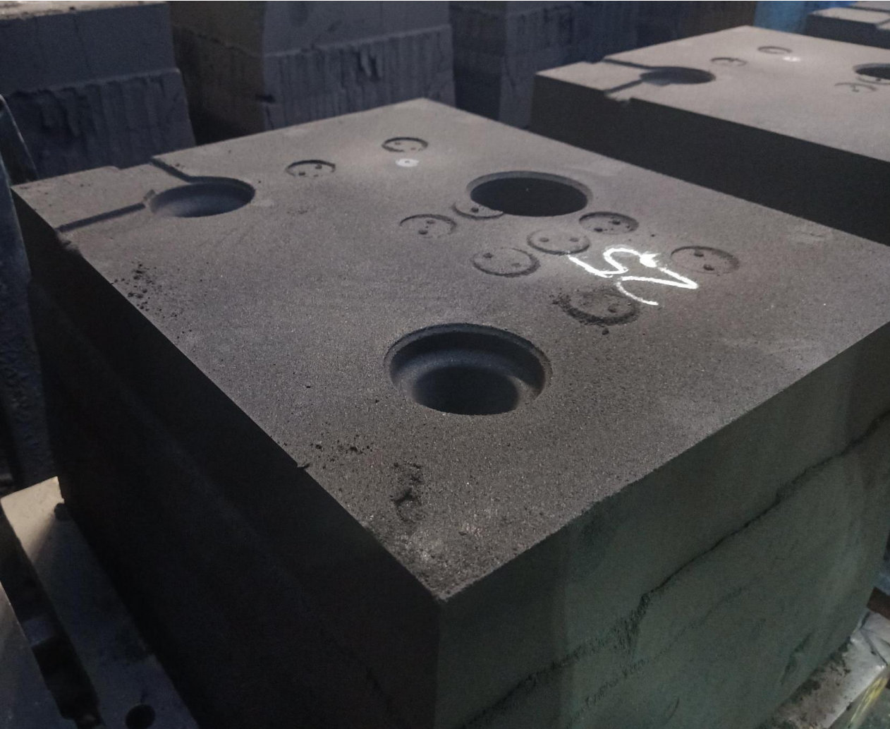
Parting line Gas Vent 0.2mm
