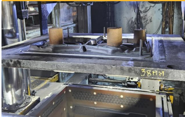
Exothermic riser on COPE side
