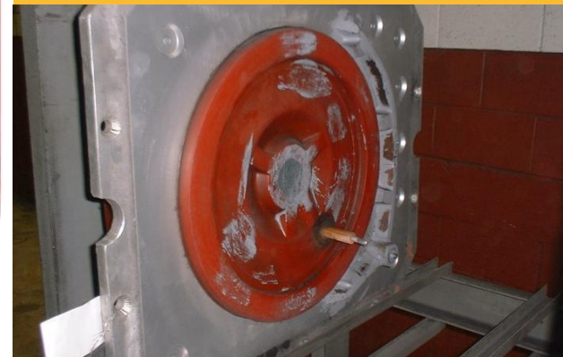
COPE side – without exothermic riser
