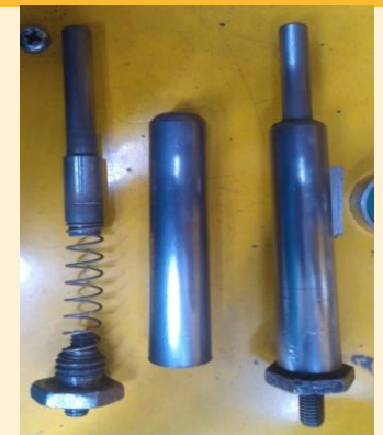
Direct vent at pattern
