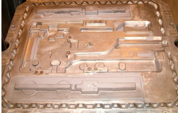
COPE side – without chills mounted
