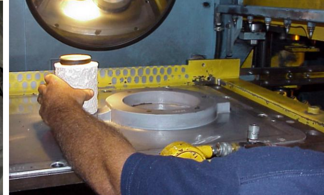
Setting of exothermic riser on COPE side
