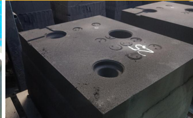
Direct vent at pattern
