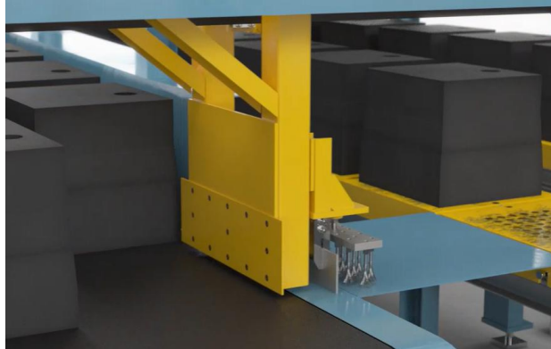
Push unit moves moulds to conveyor for extended cooling
