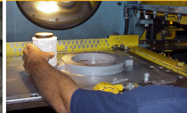
Setting of exothermic riser on COPE side
