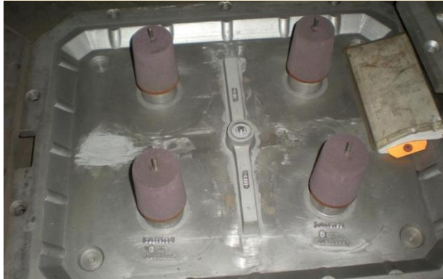
Exothermic riser on COPE side
