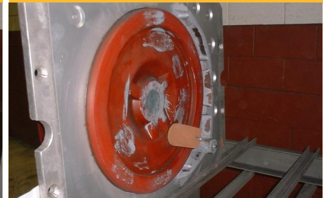
COPE side – with exothermic riser
