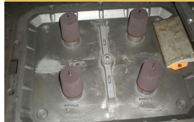
Exothermic riser on COPE side
