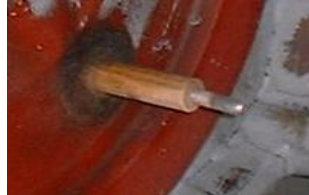
COPE side – without exothermic riser
