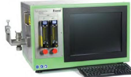
The Hot Distortion Tester is specifically designed to rapidly heat and measure any corresponding upward and/or downward deflections of a standard shell transverse sand specimen.
