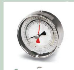
This high load gauge is used for measuring strengths up to 132 N/cm.
