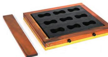
This core box makes standard specimens for tensile strength testing using self-curing (air-set) sands.
