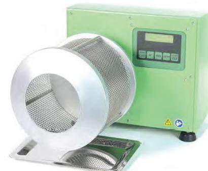
The friability of clay bonded foundry molding sand can be determined by using this instrument to measure the ability of compacted molding sand to resist abrasion or scuffing within the first few millimeters at the surface of a prepared mold.
