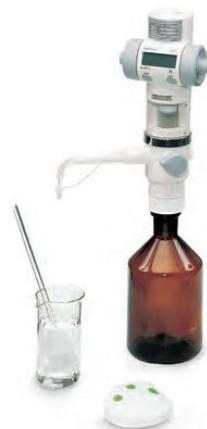
The Methylene Blue Clay Tester is used to determine the amount of live bentonite clay present in a sand sample. This instrument utilizes a magnetic stirrer for removal of the clay coating from the surface of the sand grains.
