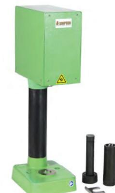
This instrument is used to prepare AFS standard sand specimens of clay bonded molding sand used for high temperature compression testing in the High Temperature Compression Tester (Model 42115).
