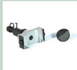
Attached to the Electronic Universal Sand Strength Machine (Model 42104), this accessory measures the transverse strength of shell/croning sand transverse specimens.
