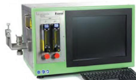
This tester measures the temperature at which shell resin coated sands melt and adhere to a heated bar. The melting temperature of the sand is considered the melt point or stick point.
