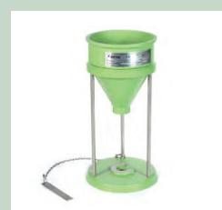
This accessory is required to fill the specimen tube for compactability tests. It assures that properly riddled sand fills the specimen tube from a standard and fixed distance.
