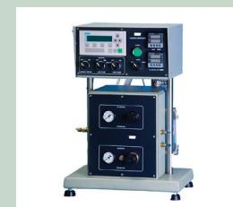
The vaporizer connects to the Test Pieces Blower (Model 42109) in order to control the gassing and purging sequence of the test specimen.
