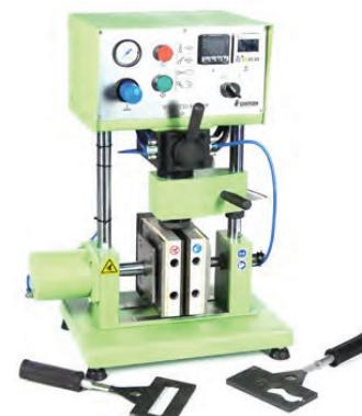
This instrument is used to make standard tensile strength, shell transverse and hot distortion test specimens.
