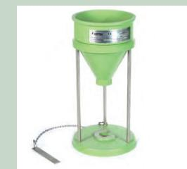
This accessory assists in filling the specimen tube for compactability tests. It assures that properly riddled sand fills the specimen tube from a standard and fixed distance. Both the Digital Pneumatic Sand Squeezer (Model 42160) and the Sand Rammer (Model 42100) use this accessory.
