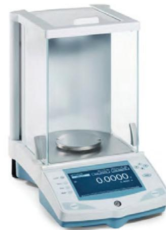
This high precision weighing instrument is necessary for standard tests requiring high accuracy measurements.
