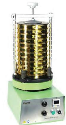
The sifter is used to determine the grain fineness and distribution of foundry sands.
