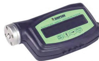
Mold hardness is the resistance offered by the surface of a prepared sand mold to be penetrated by a loaded plunger. Both the Mold Hardness Tester B-Scale (Model 42142), which uses a ball penetrator, and the Mold Hardness Tester C-Scale (Model 42143), which uses a conical penetrator, are handheld devices that measure the depth of penetration into a mold surface of a plunger. The C-Scale hardness tester is suitable for molds having hardness readings over 90.
