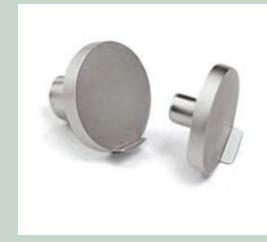
This accessory is attached to the Universal Sand Strength Machine (Model PFG) to measure splitting strength. This test is considered an indirect measurement of a clay bonded molding sand's tensile strength property.
