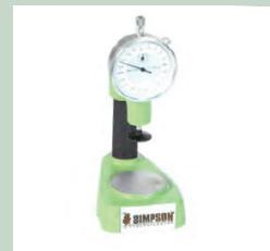
This accessory measures the deformation of a clay bonded sand specimen after a compression strength test is done on the Electronic Universal Sand Strength Machine (Model 42104). Deformation is the change in the length of the sand specimen before and after the compression test.
