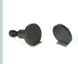
This accessory is attached to the Electronic Universal Sand Strength Machine (Model 42104) to measure splitting strength. This test is considered an indirect measurement of a clay bonded molding sand's tensile strength property.
