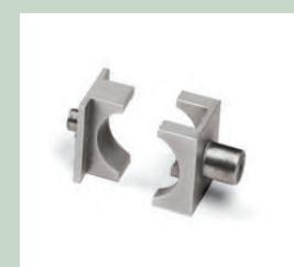
To measure the twin-transverse shear strength of clay bonded molding sand specimens, these two uniquely designed testing clamps are mounted to the Universal Sand Strength Machine (Model PFG).
