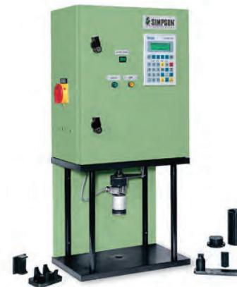
This multi-purpose instrument is used to determine strength properties of clay and/or chemically bonded sand specimens. The Minilab may be used to create a 50mm x 50mm cylindrical test specimen and can run many different sand strength tests using additional accessories. These tests include: compactability, compression strength, splitting strength, twin-transverse shear strength, core transverse (bending) strength and core tensile strength.
