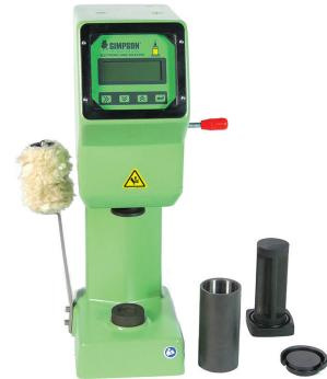
This sand squeezer is used to prepare standard AFS 2" x 2" (50mm x 50mm) sand specimens and to determine the compactability of prepared clay bonded molding sand. The instrument can be a replacement for the standard 3-ram method of making sand specimens using a traditional sand rammer.
