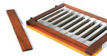
This core box makes standard specimens for transverse strength testing using selfcuring (air-set) sands.
