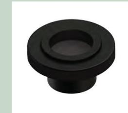
This accessory determines permeabilities of core or mold coatings imparted upon the included screens.
