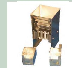
This accessory is used to prepare a 125 gram or smaller representative sample of unbonded foundry sands for sieve analysis testing.
