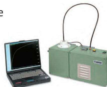
This instrument can be used to accurately measure the gas pressure generated over time from a foundry sand sample heated to a set temperature.
