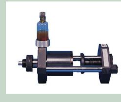
This accessory is a force multiplier that, when used with the Electronic Universal Sand Strength Machine (Model 42104), can perform a compression strength test on a standard AFS 2" x 2" (50mm x 50mm) sand specimen with a compression strength range of 250–3100 PSI (170–210 N/cm<sup>2</sup>).
