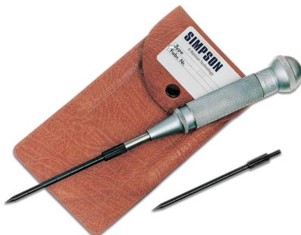
This handheld tester determines the degree of curing in lower zones of chemically bonded molds and cores. In addition to identifying curing time, it is useful in determining the proper strip time.
