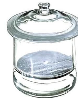
The desiccator is used to protect sand specimens from water vapor in the air during the cooling of samples after those samples have been heated in the Muffle Furnace (Model 42127).
