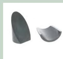
This test is used to determine the flowability of a molding sand.
