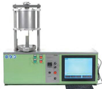
The High Temperature Compression Tester is used to determine the hot strength properties of a molding sand sample. The instrument measures both hot compressive strength and hot deformation.
