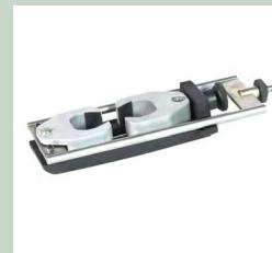
When mounted to the Electronic Universal Sand Strength Machine (Model 42104), this accessory measures the cold tensile strength of standard dog bone specimens prepared from cold box, core oil, hotbox/warmbox and nobake/air-set sands.
