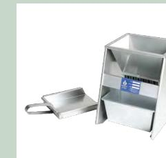
When used in conjunction with the Microsplitter (Model 42106B), this accessory is used to prepare a representative sample of unbonded foundry sands for sieve analysis testing. Fourteen (14) 1/2" chutes divide the sand accurately in half to provide representative sand samples down to 125 grams.
