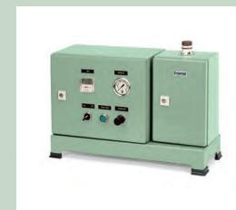
This equipment controls gassing of test specimens for gas-cured molding sand.
