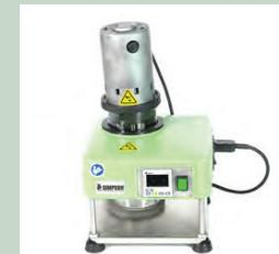
The Rapid Sand Washer is used to ensure correct and repeatable test results when preparing sand samples for the AFS Clay Tester (Model 42131). This sand washer uses highspeed agitation to remove all clay from the sand grains within the molding sand sample.
