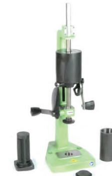
The Sand Rammer is used to prepare standard AFS 2" x 2" (50mm x 50mm) cylindrical sand specimens. It is also used to determine the compactability of prepared clay bonded molding sand used in a foundry.
