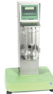
The AFS Clay Tester is used to determine the percentage of particles with a diameter less than 20 microns in a foundry sand sample.
