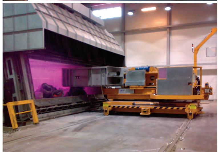
**Charging Machines, rail mounted, for charging dry hearth, stationary and tilting furnaces in rapid and precise way**
