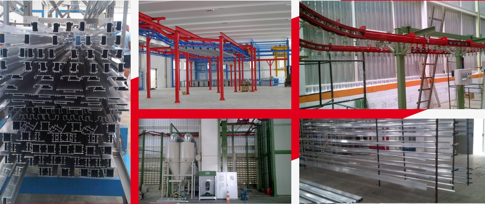
Over the years **Cisart** developed several configuration powder coating plants, each **tailored over a specific** customer **need**. The pretreatment cycles and the chemical specification are established in agreement with major worldwide chemical specialty suppliers. The main plant configurations are:
