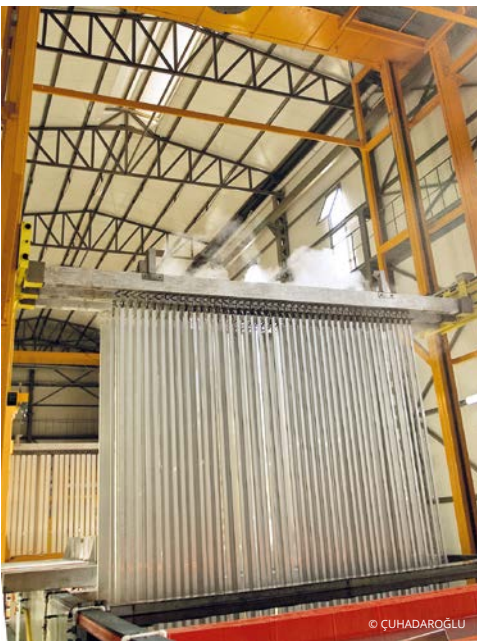
Most pre-treatment operations, including degreasing and chemical etching, are carried out in shared tanks.
